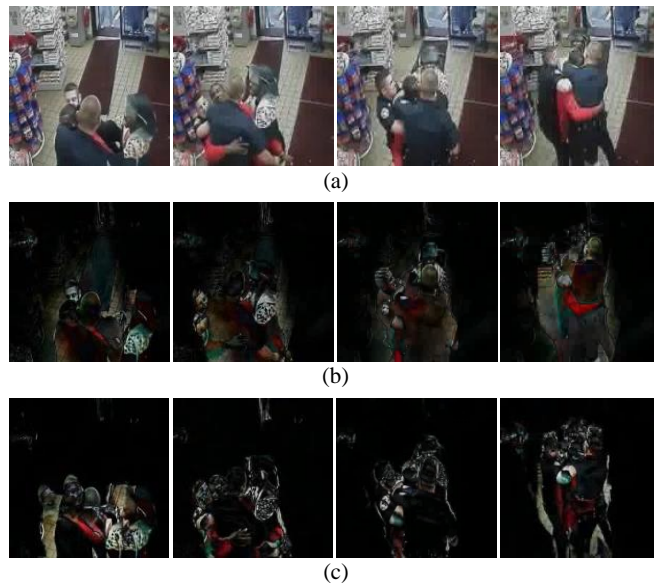
Figure 3.2: Input pre-processing for the proposed model. (a) shows key-frames of an example video clip. (b) demonstrates the effect of performing background suppression on video frames of (a). The last row (c) shows time-steps of the frame difference derived from the video clip of (a).
