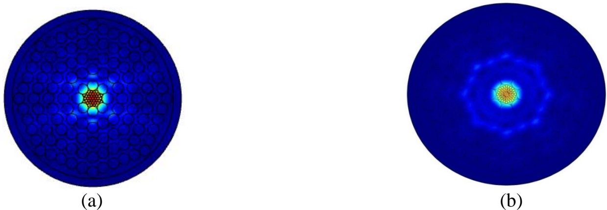
Fig 2.5 Power flow distribution of (a) low confinement loss (b) high confinement loss designs
