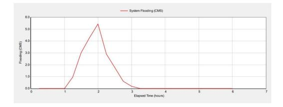
Figure 27: System flooding for 5yr return period with LID
