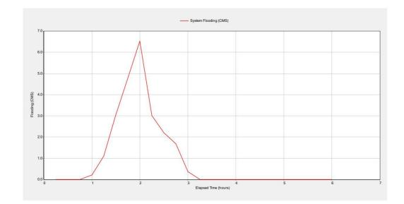
Figure 28: System flooding for 10yr return period without LID
