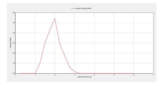
Figure 26: System flooding for 5yr return period without LID
