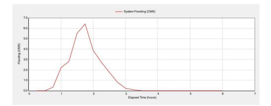
Figure 31: System flooding for 25yr return period with LID
