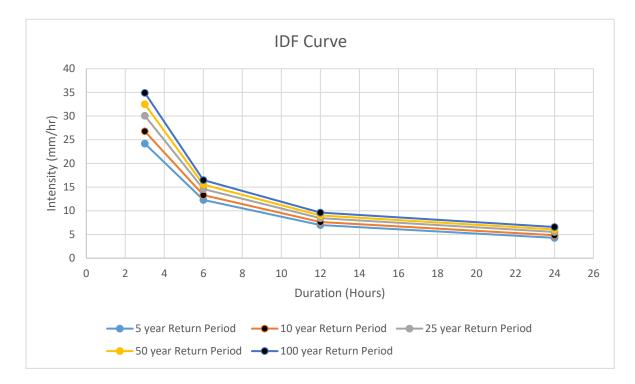
*Figure 9: Intensity-Density-Frequency curve by Gumbel's Distribution for different return periods.*
