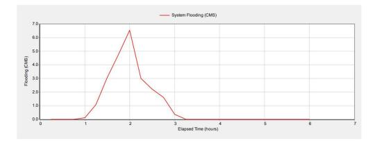
Figure 29: System flooding for 10yr return period with LID
