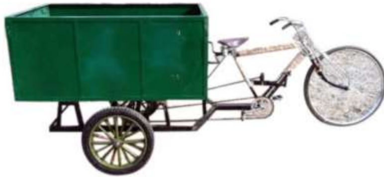
Figure 4:12 Existing collection vehicle type with single compartment to collect waste from household
