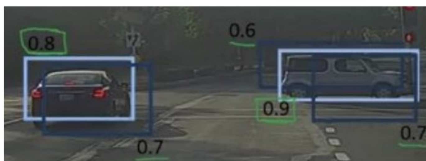
Figure 3.6: Selecting the Next Box with the Highest Score and Taking IoU
