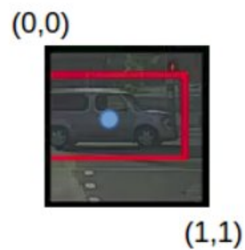
Figure 3.7: Setting the Midpoint of a Bounding Box
