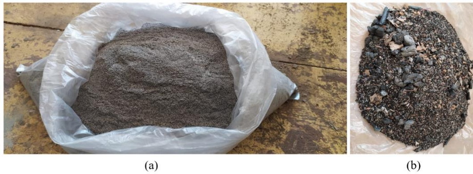
Figure 16: (a) Burned RHA after the filtering (b) Leftovers after the filtration
