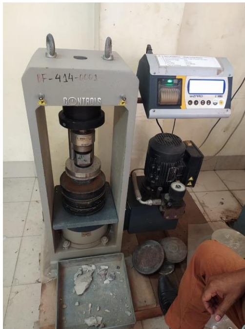
Figure 11: During Compression test for B-S-RHA5 in the Compression-Flexural Testing Machine
