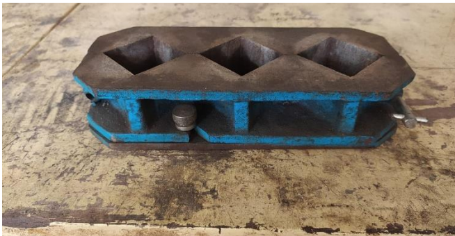
Figure 8: Mold for setting the blocks
