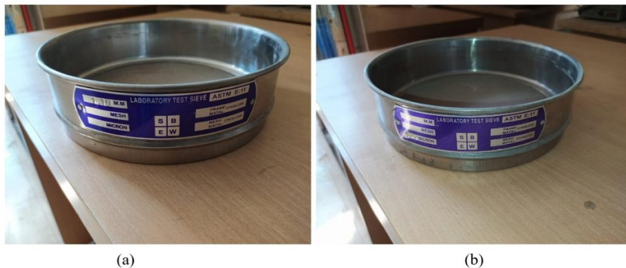
Figure 15: Sieve used for filtration process (a) 1.18 mm (b) 600 microns
