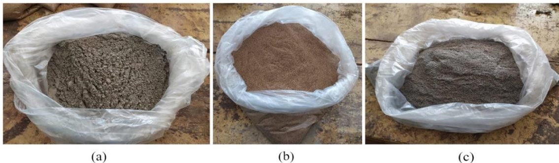
Figure 13: Elements used for making the cylindrical block (a) Cement (b) Sand (c) Rice Husk Ash
