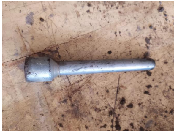
Figure 22: Hammer for pushing the mixture inside the mold
