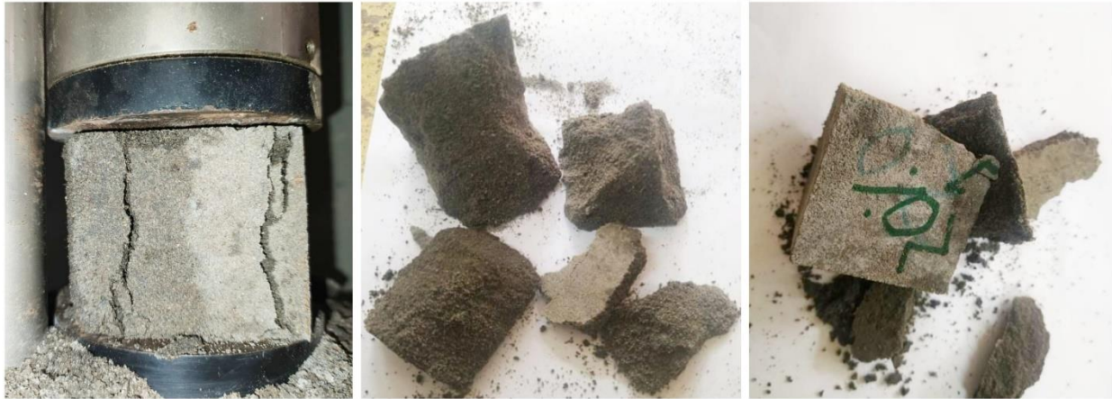
Figure 12: B-S-RHA20 after the compression test
