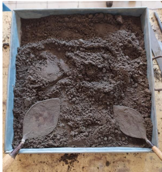
Figure 20: Mixture of the elements after the hand mixing using hand-shovels
