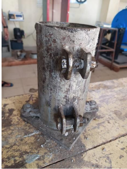
Figure 21: Mold for setting cylindrical block
