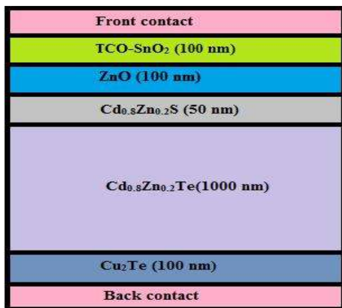
Fig. 3.2 Schematic diagram of the proposed solar cell
