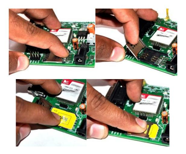
*Warning:* Be careful about SIM card slot as it is too delicate one while inserting in and removing out SIM card.
