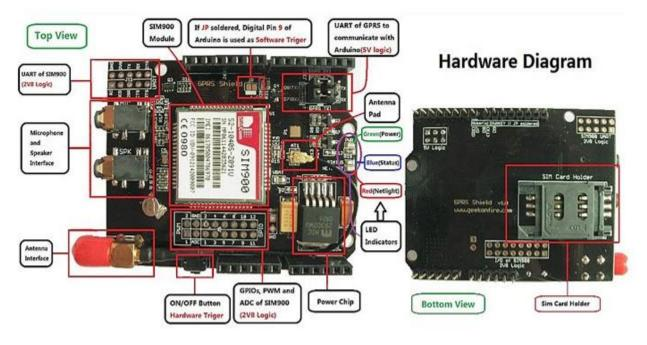
GSM (Global System for Mobile) / GPRS (General Packet Radio Service) TTL –Modem is SIM900 Quad-band GSM / GPRS device, works on frequencies 850 MHZ, 900 MHZ, 1800
