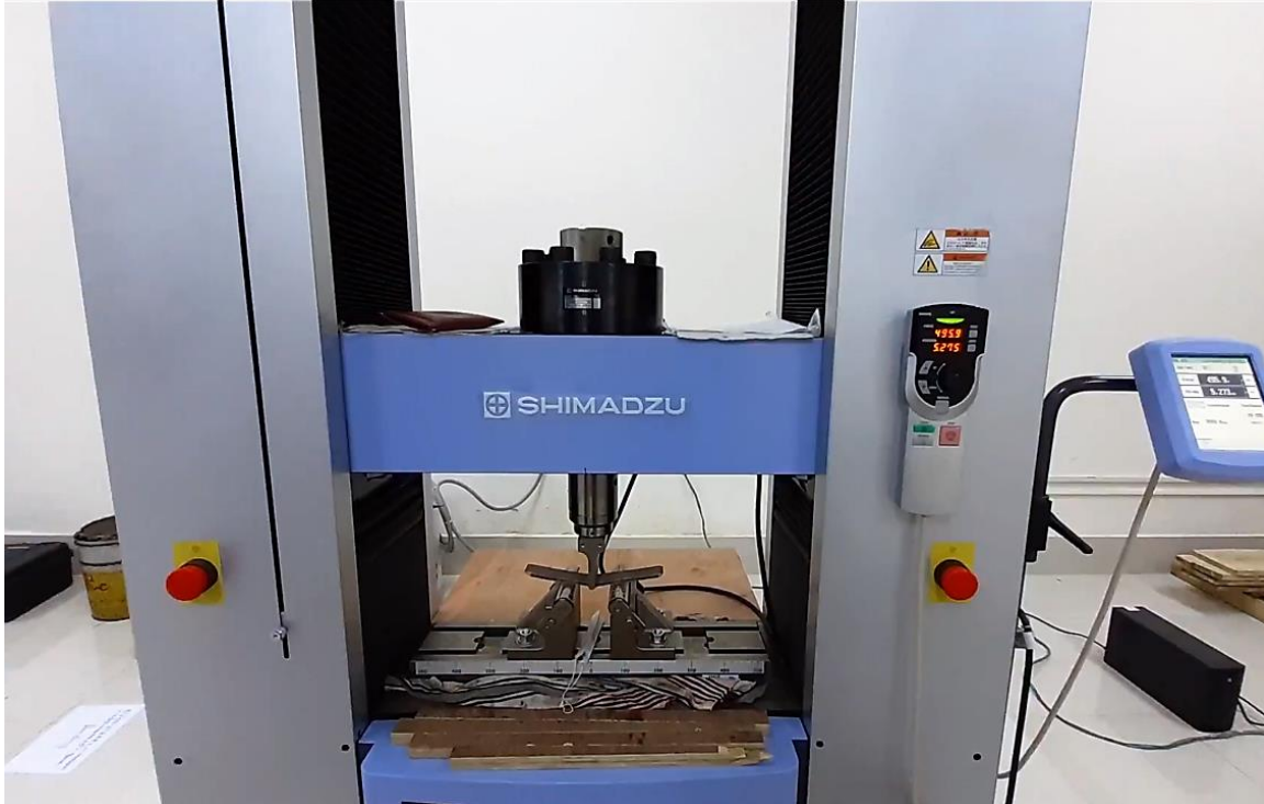
Figure 3.10 Flexural testing equipment with the specimen
