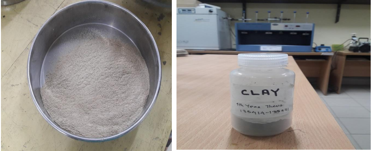
Figure 3.3.2. Clay preparation for obtaining turbidity in Type 2 water
