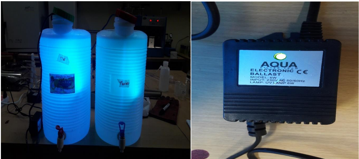
Figure 3.5. UV experiments and the electric ballast of UV lamps
