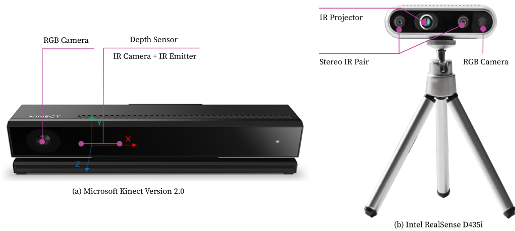
FIGURE 2.2: Example of RGB-D camera for depth information acquisition (a) Microsoft Kinect V2 (b) Intel RealSense D435i
