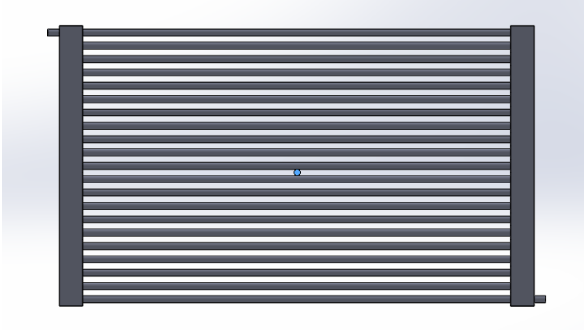
Figure 2: Car radiator with 21 numbers of pipes
