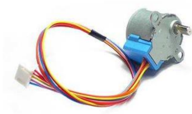
Figure 2.13 28BYJ-48 Unipolar Step Motor
