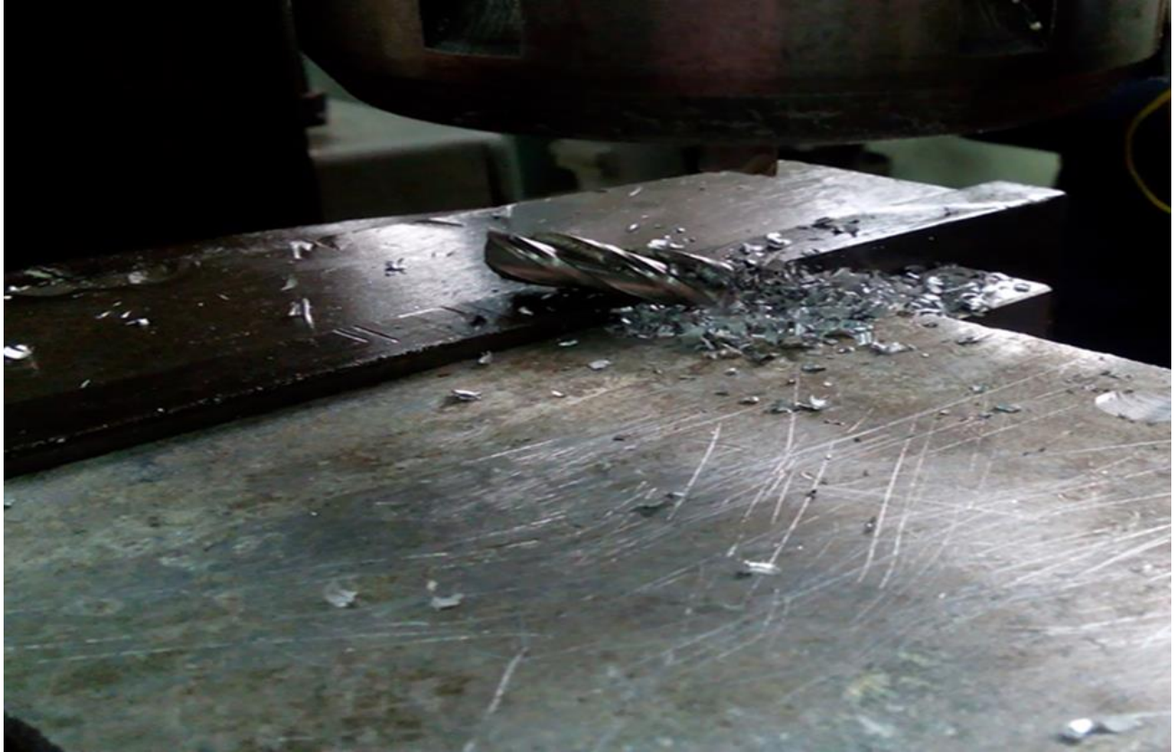
Figure 1: Damage of cutting tool in dry machining during our experiment
