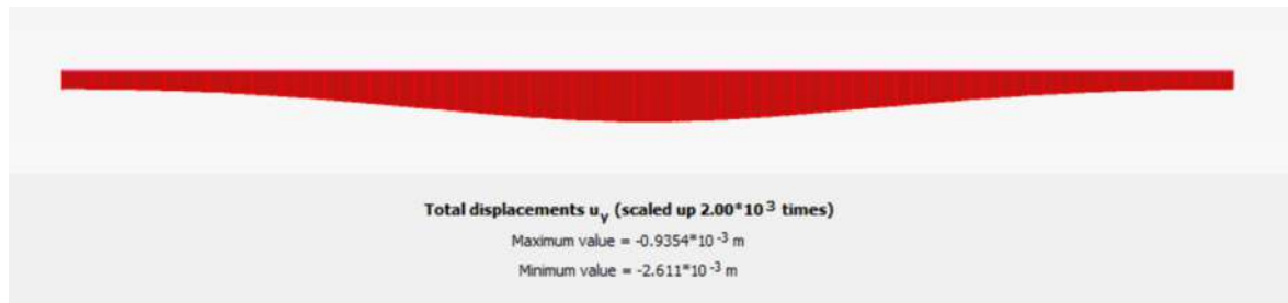
Figure 31: Excavation induced Settlement (#1A, 55m depth, GWL=-20m)
