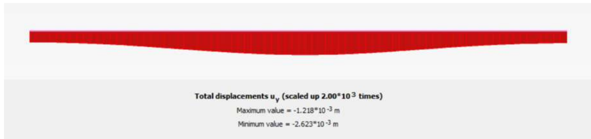
Figure 39: Excavation induced Settlement (#1A, 65m depth, GWL=-20m)
