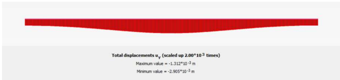
Figure 43: Excavation induced Settlement (#1A, 65m depth, GWL=-60m)
