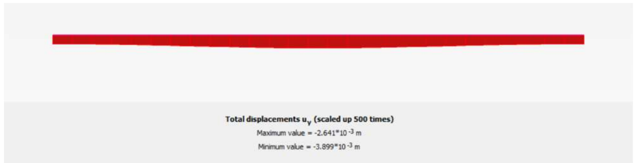
Figure 91: Excavation induced Settlement (#2A, 50m depth, GWL= -60m)
