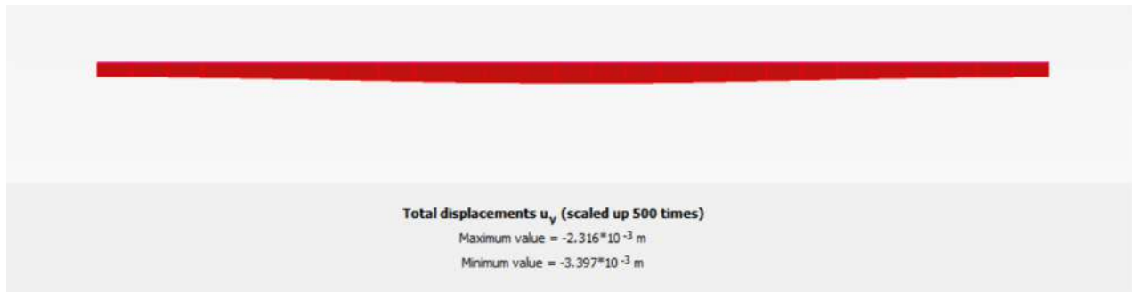
Figure 87: Excavation induced Settlement (#2A, 50m depth, GWL= -20m)
