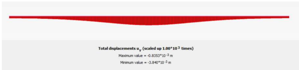
Figure 27: Excavation induced Settlement (#1A, 45m depth, GWL=-60m)
