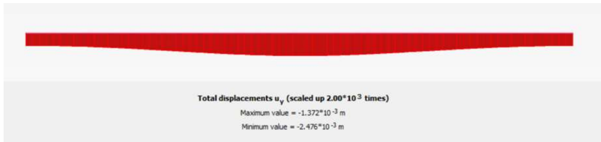
Figure 51: Excavation induced Settlement (#1A, 75m depth, GWL=-60m)
