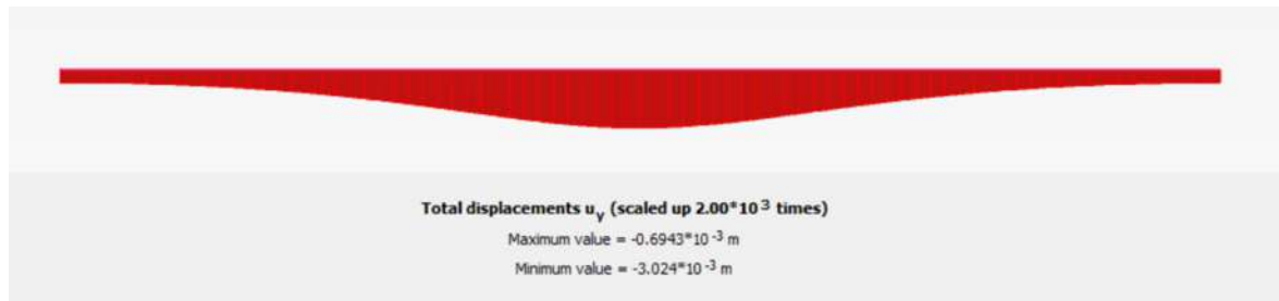
Figure 23: Excavation induced Settlement (#1A, 45m depth, GWL=-20m)
