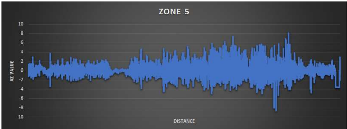
Figure 4-12: average Z axis acceleration versus distance for zone 5
