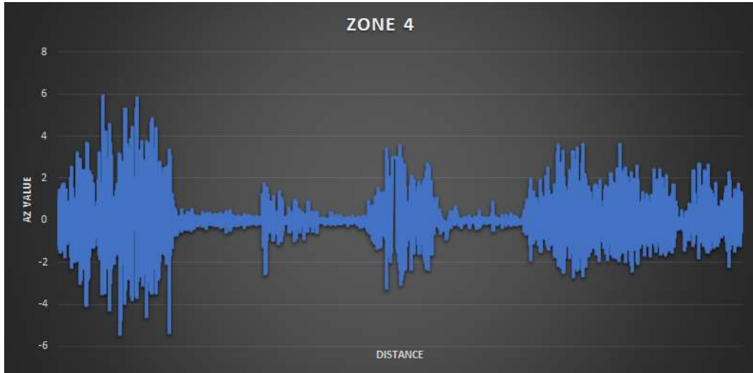
Figure 4-10: average Z axis acceleration versus distance for zone 4
