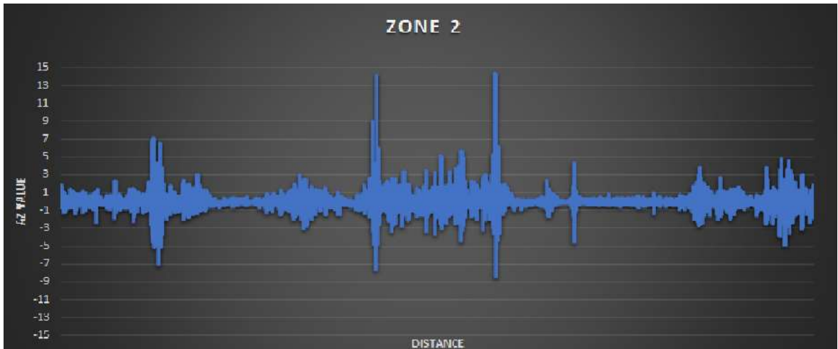
Figure 4-7: average Z axis acceleration versus distance for zone 2
