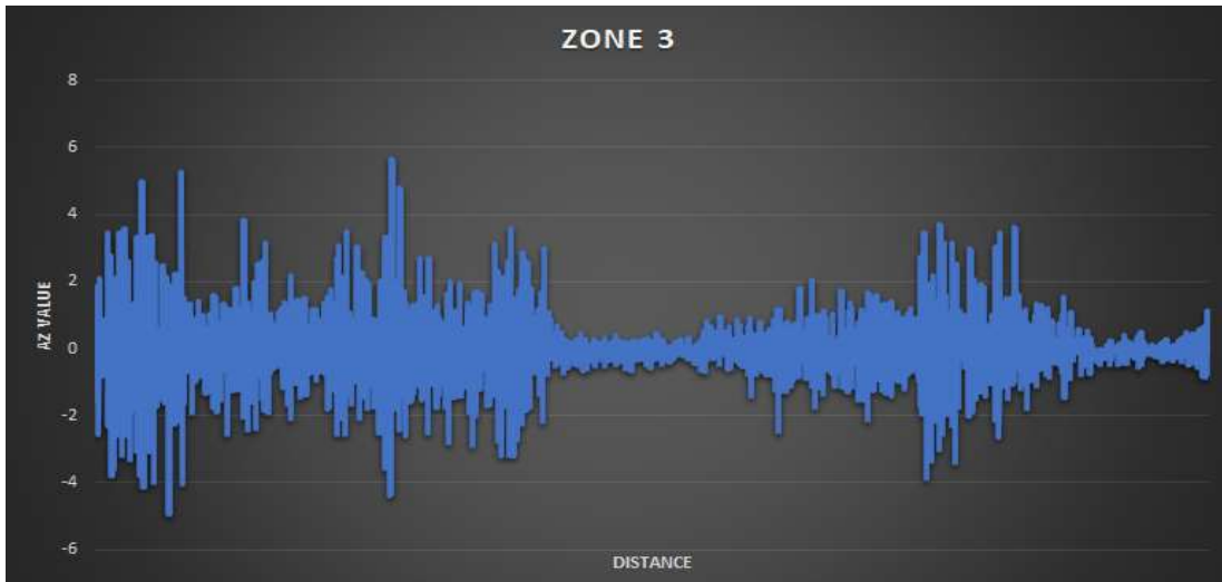
Figure 4-9: average Z axis acceleration versus distance for zone 3
