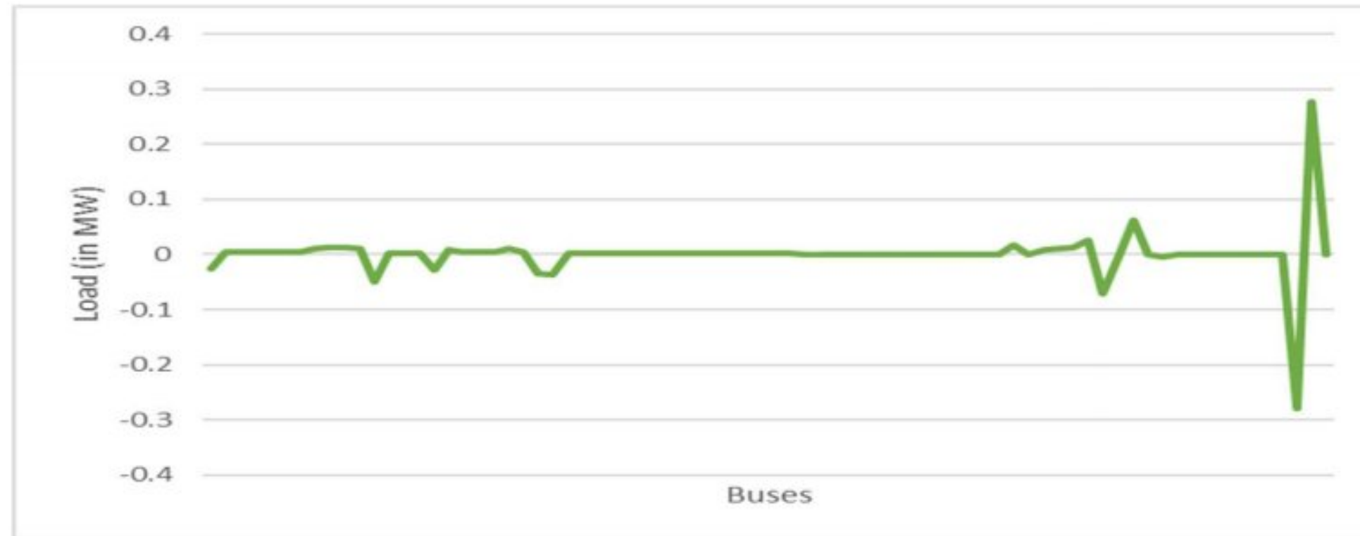
Figure 5.35: Line plot showing the variation of load (in MW unit) of each of the buses in the substation of IUT (by taking a portion of the table generated)
