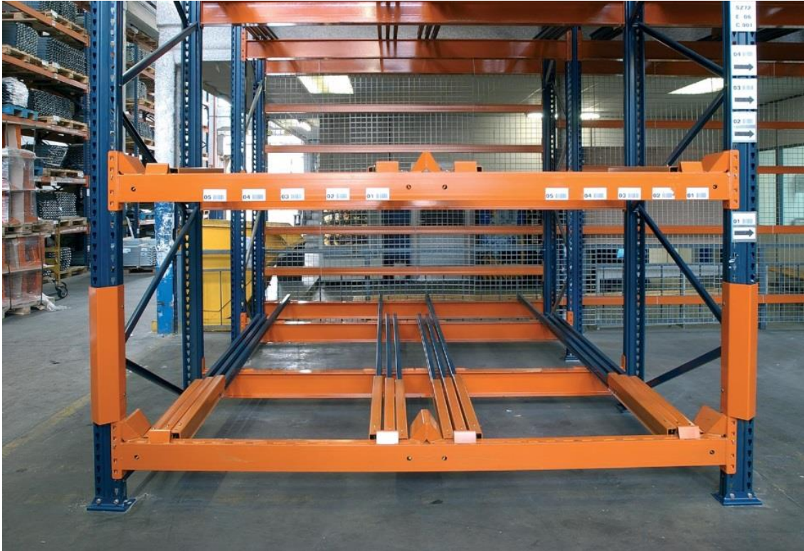
Figure 2.8 Push Back Pallet Racking
