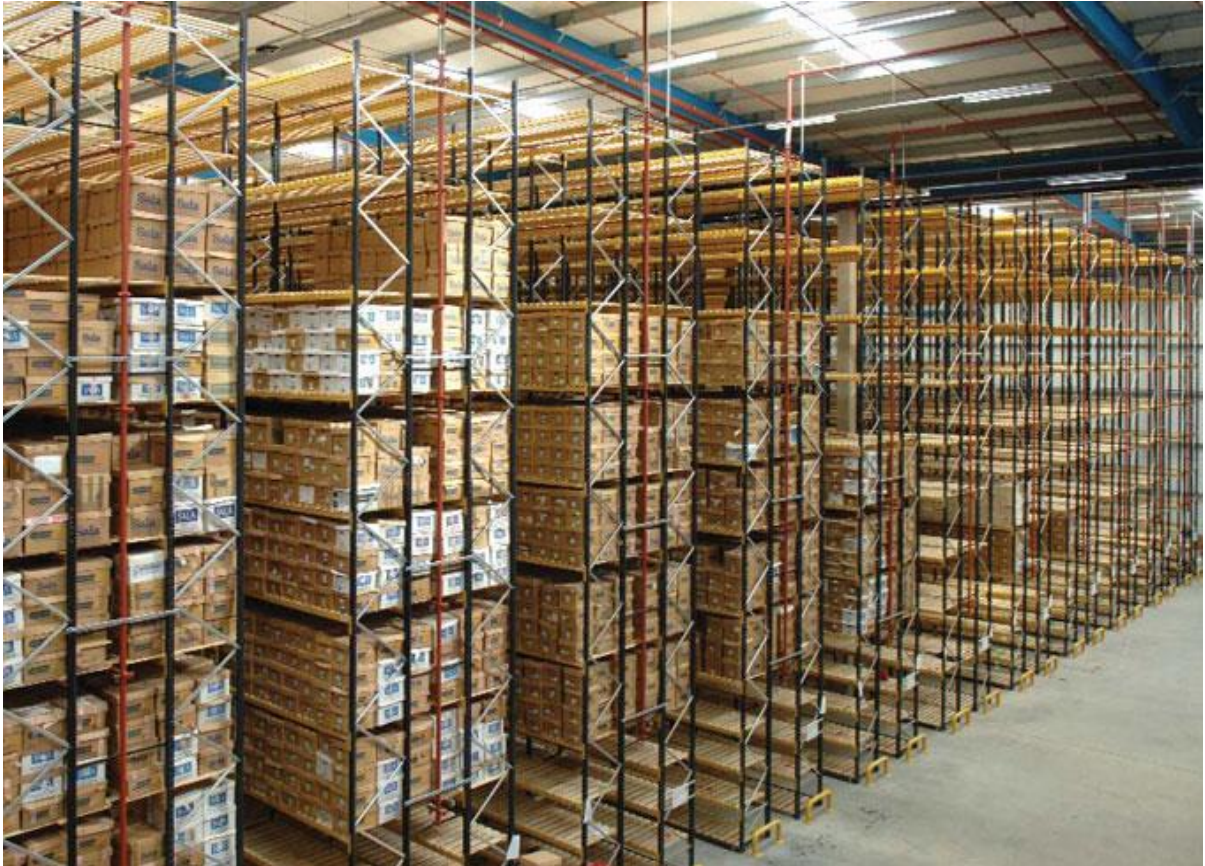
Figure 2.7 Adjustable Pallet Racking
