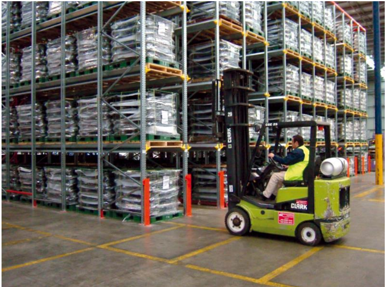
Figure 2.6 Drive-In Pallet Racking
