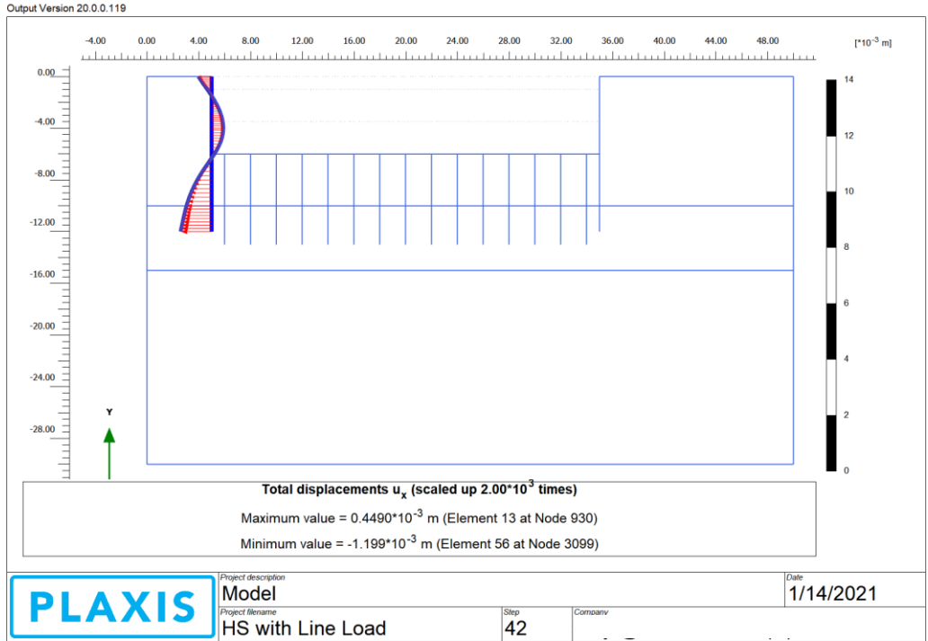
Figure 5.3.12: Maximum wall displacement for HS Model with adjacent load (wall thickness 1m)
