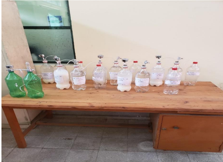
Figure 13 Installation Of 5 Setups of Rice Waste In 5 Different Ratios (1:1,1:2,1:3,1:4,1:5) In the Lab
