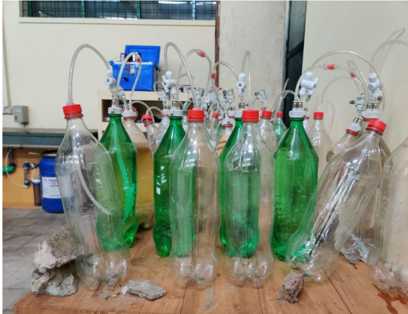
Figure 20 Setups Modified Using One Way Check Valves
