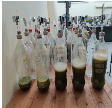
Figure 16 Installation Of 5 Setups of Vegetable Peel Waste,5 Different Ratios (1:1,1:2,1:3,1:4,1:5) In the Lab
