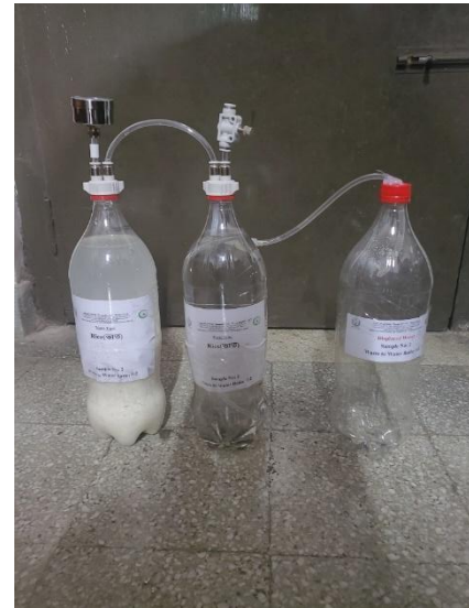
Figure 12 First Experimental Setup Using Three Bottles for Aerobic Digestion and Water Displacement
