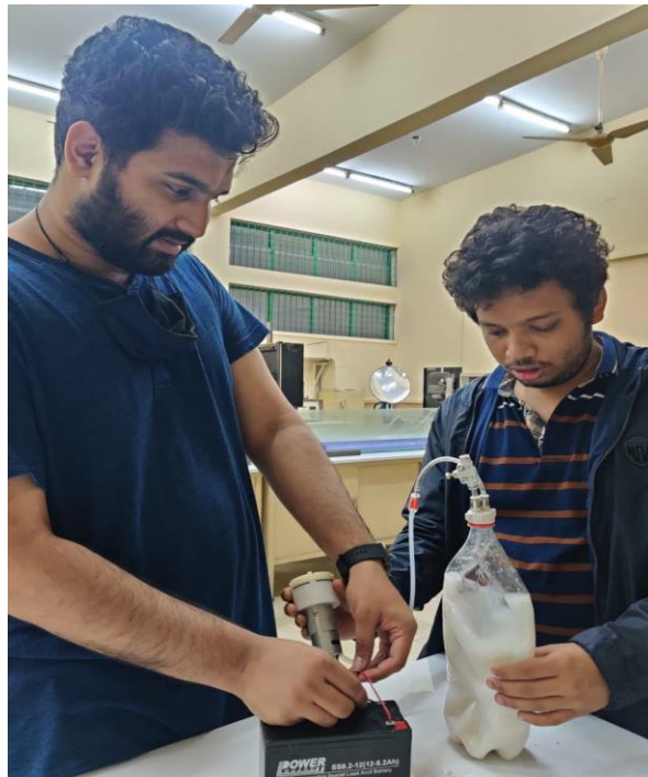
Figure 21 Using Suction Machine to Create Anaerobic Condition
