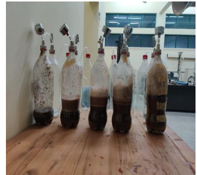
Figure 17 Installation Of 5 Setups of Potato Peel Waste,5 Different Ratios (1:1,1:2,1:3,1:4,1:5) In the Lab
