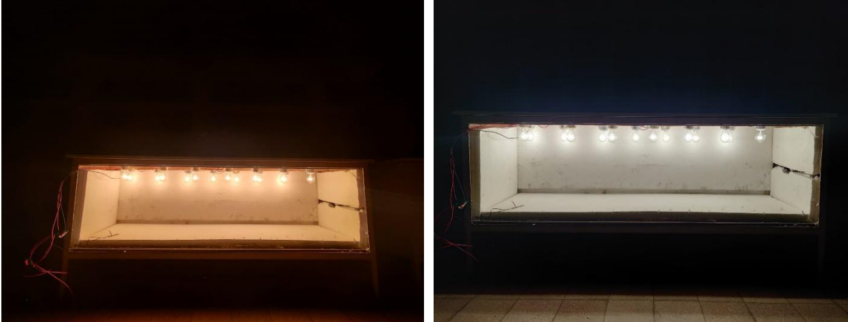
Figure 28 Construction of An Incubator for Maintaining Temperature of Mesophilic Condition in Winter Time
