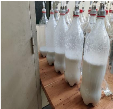
Figure 15 Installation Of 5 Setups of Rice Waste,5 Different Ratios (1:1,1:2,1:3,1:4,1:5) In the Lab
