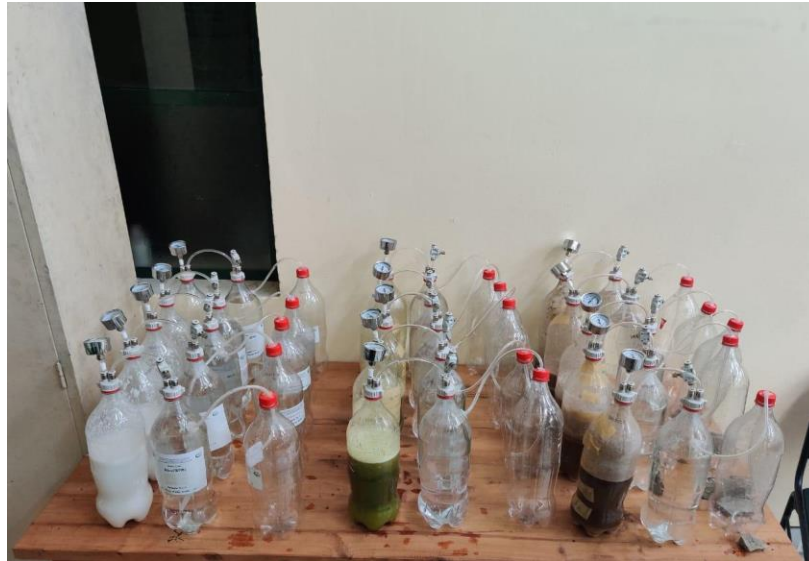
Figure 14 Installation Of 15 Setups of Rice Waste, Vegetable Peel Waste and Potato Peel Waste In 5 Different Ratios (1:1,1:2,1:3,1:4,1:5) In the Lab
