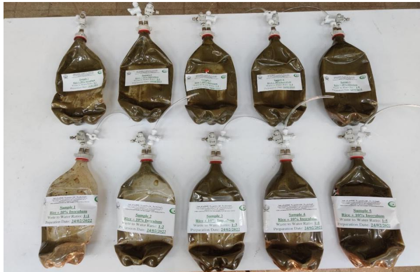
Figure 29 Preparation Of 4th Batch of Rice Waste With 10% And 20% Inoculation With (H.D) In Different Ratios (1:1, 1:2, 1:3, 1:4, 1:5)
