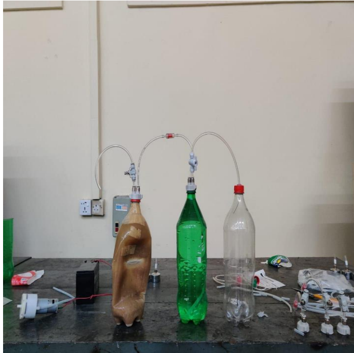
Figure 22 Three Bottle Setup with One Way Check Valve and First Bottle in Anaerobic Condition
