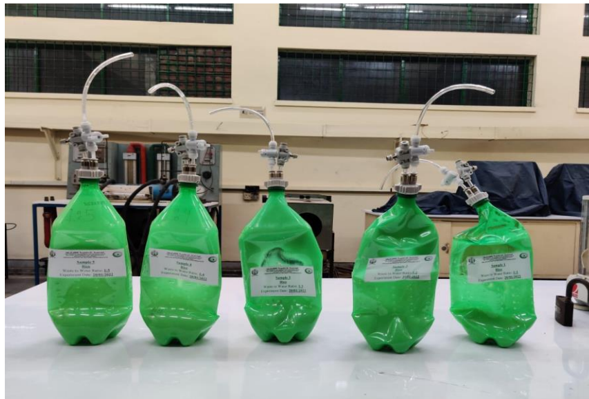
Figure 26 Single Bottle Setup Using Trimmer Valve and Switch Valve at The Openings
