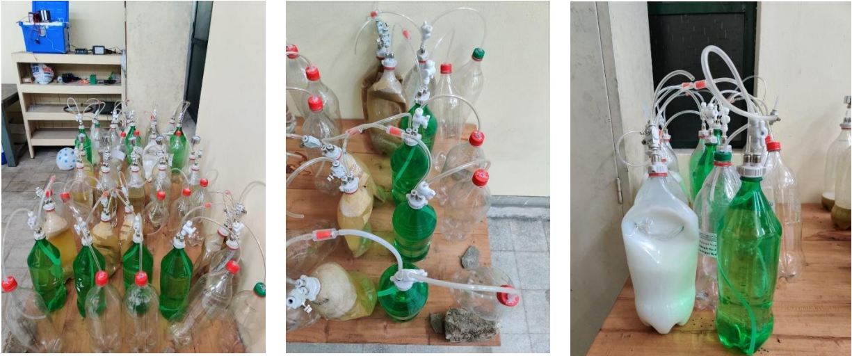
Figure 23 Installation Of 5 Setups of Rice, Vegetable Peels, Potato Peel Waste In 5 Different Ratios (1:1,1:2,1:3,1:4,1:5) In the Lab After Modifications and Alterations in The Setups
