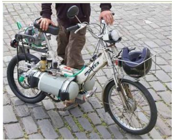
Fig 2.1: compressed air vehicle model
