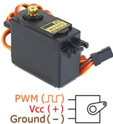
Fig 3.12: Servo motor pinout
