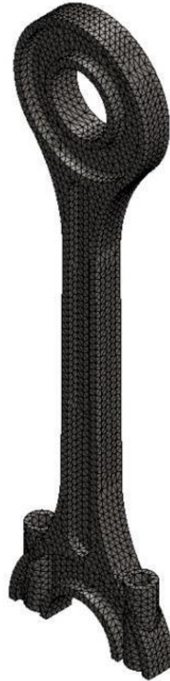
Figure 8: The model after mesh is generated
