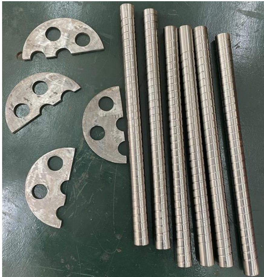
Fig. Machined corrugated tubes and baffles.
