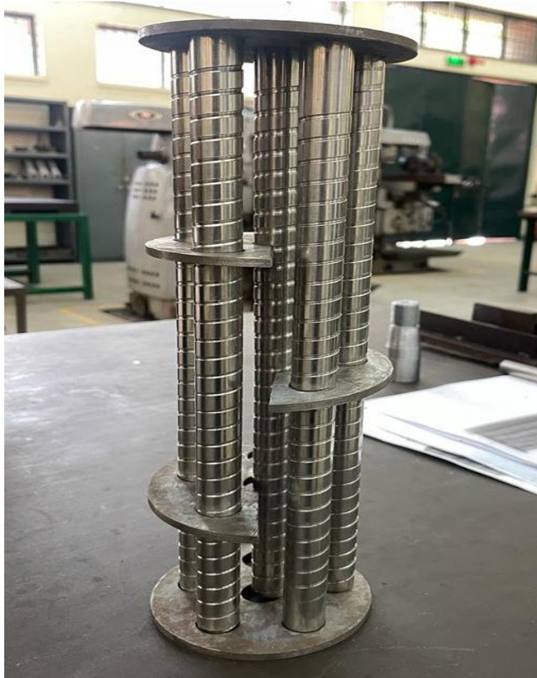
Fig. Spiral Tubes and baffles arrangement.
