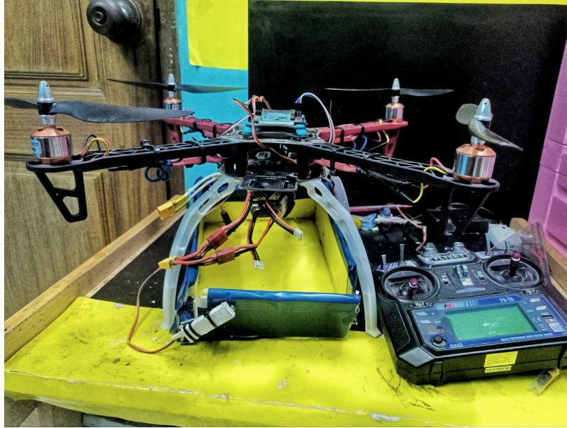
Figure 44: Firefighting quadcopter prototype with dropping mechanism
