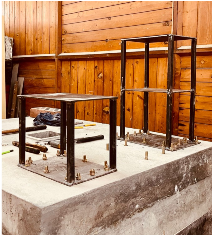
(a) Final structure fixed to base
