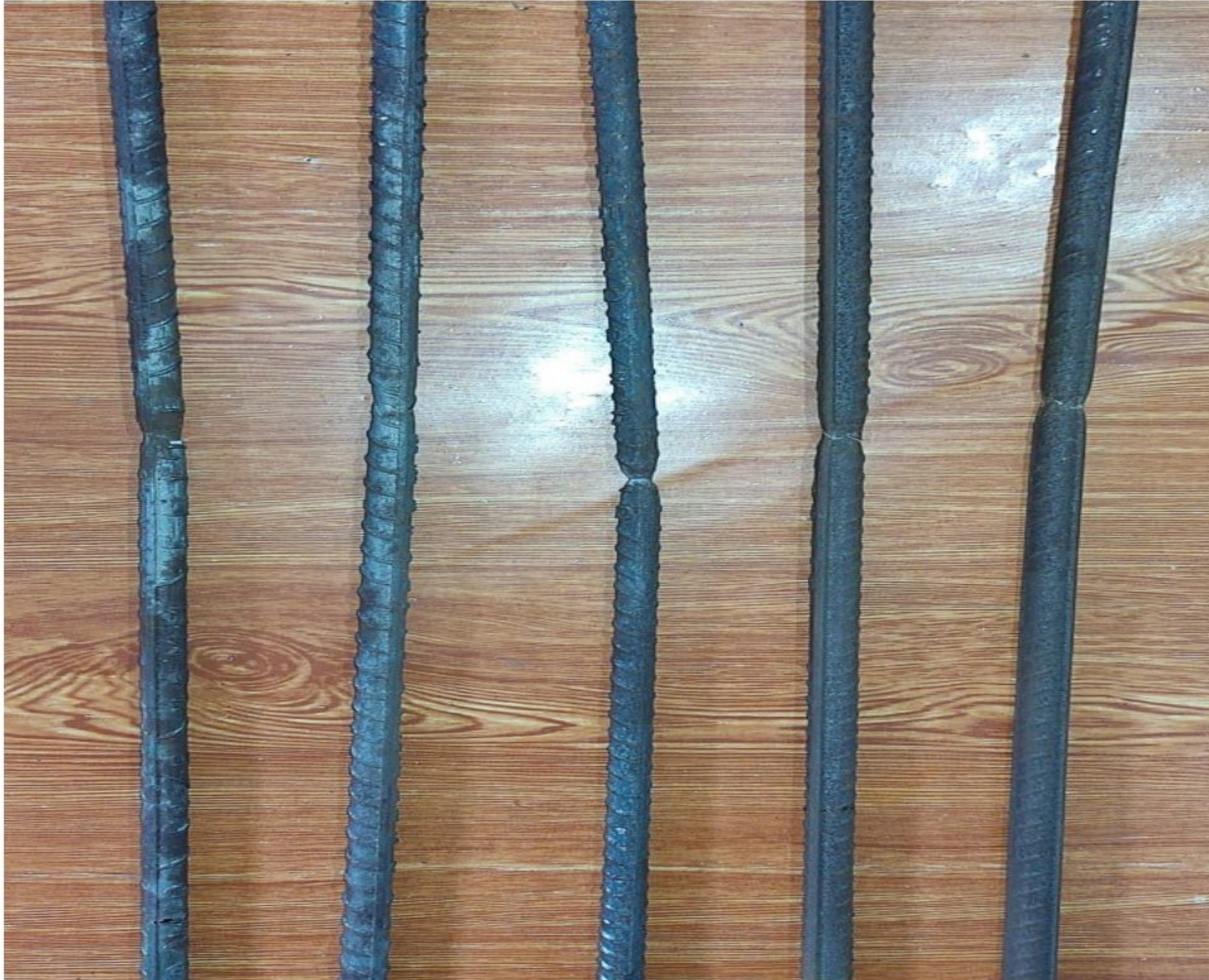
Fig 3.2: Necking before fracture
