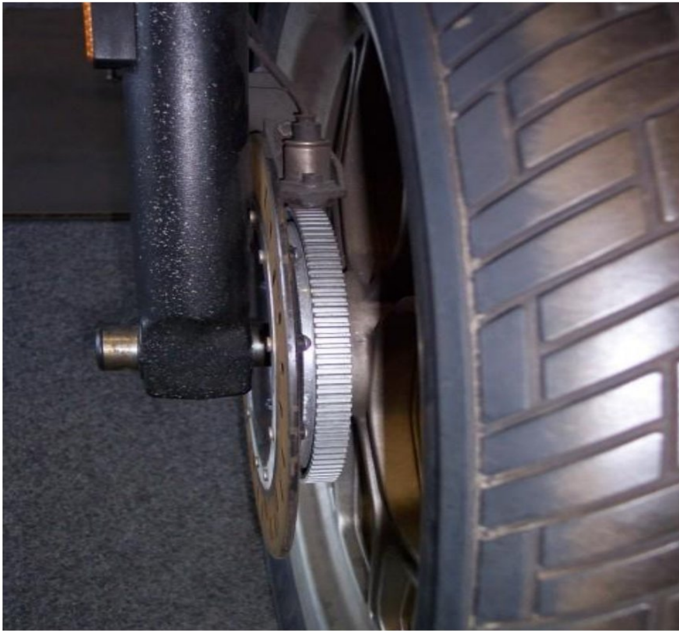
Figure 8 Toothed-wheel ABS sensor on a BMW K75 motorcycle
