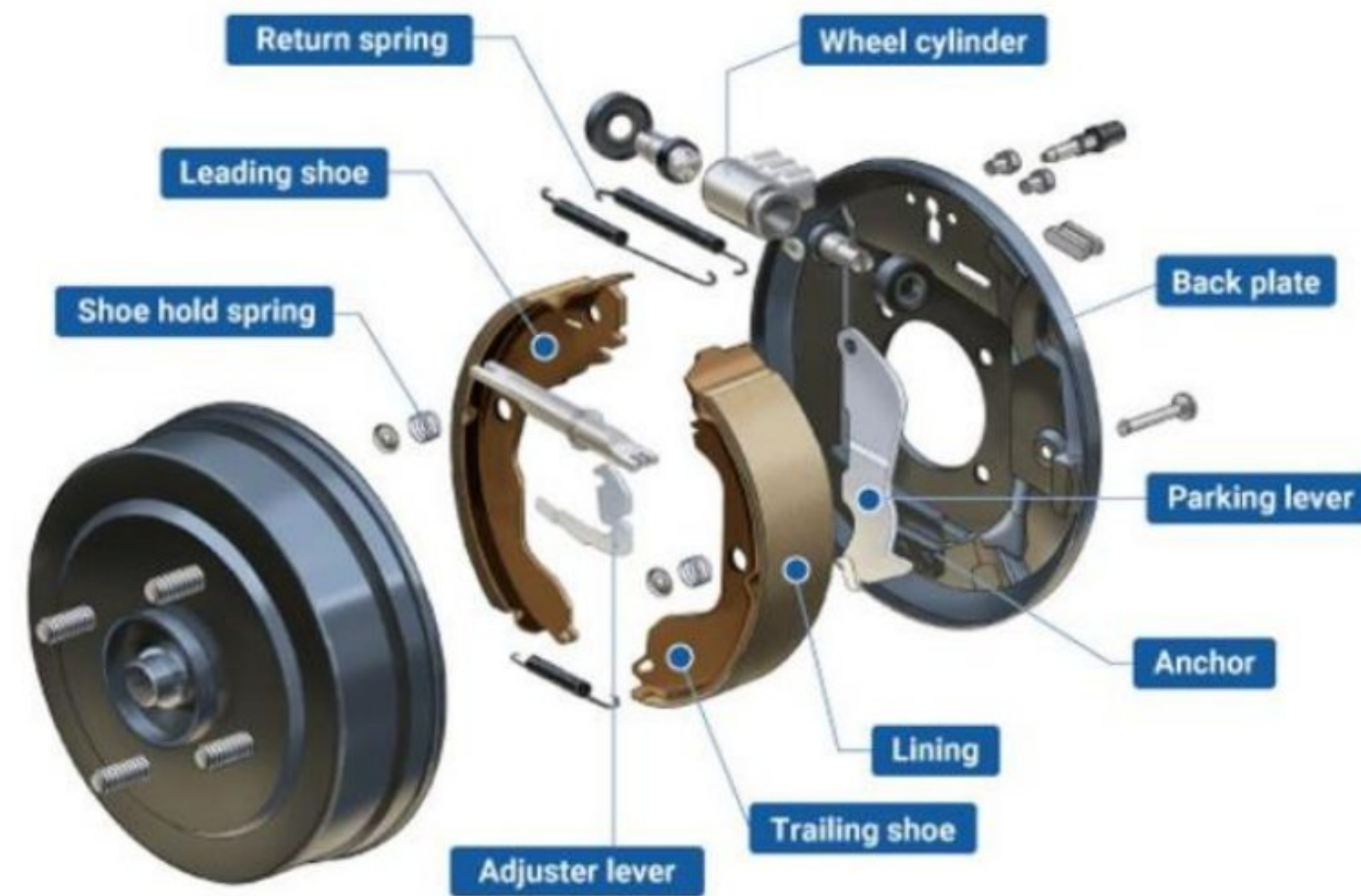
Figure 2 Components of Drum Brake
