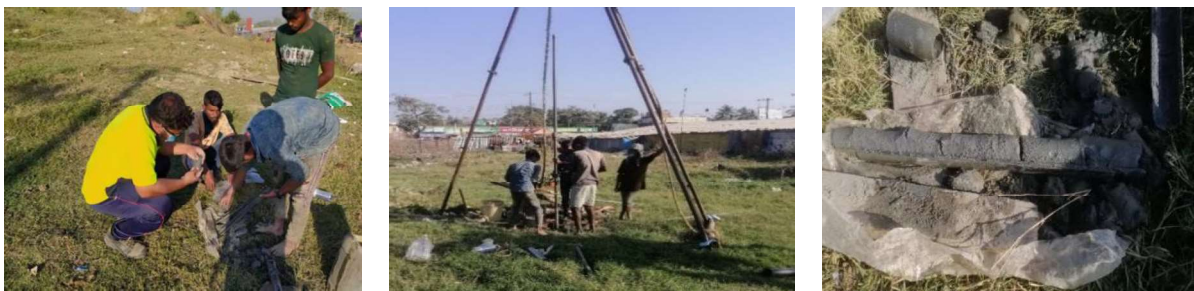
Figure 3.2. Soil Sample Collection
