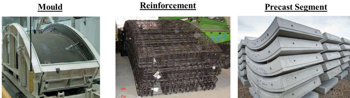
Figure 2.12 Segmental Lining Construction
