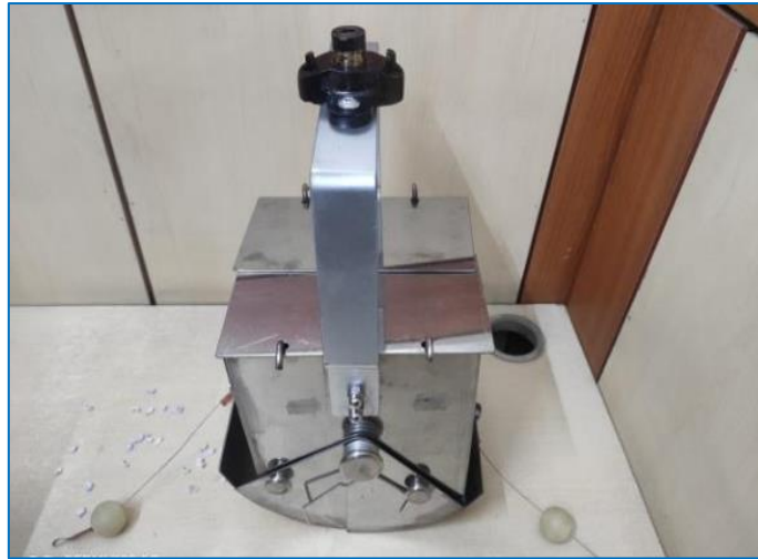
Figure 3.3: Ekman grab sampler used for sediment samples collection in this study.
