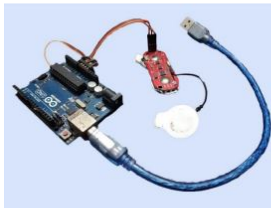
FIGURE 3.2: EMG-based module to capture EMG signals from the patient's arm
