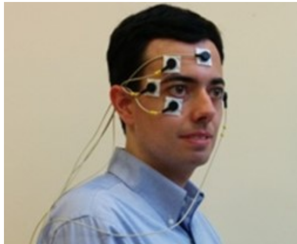
Figure 2.8: Placement of electrodes for Electrooculogram (EOG) signal acquisition (image adopted from [93]).
