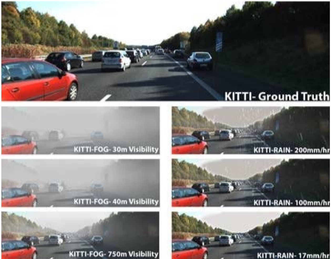
Figure 9: Fog and rain augmentation from the paper implementation "Robustness of Object Detectors in Degrading Weather Conditions" [9]
