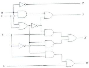
Figure 1: A logic circuit for Question 2.b)
