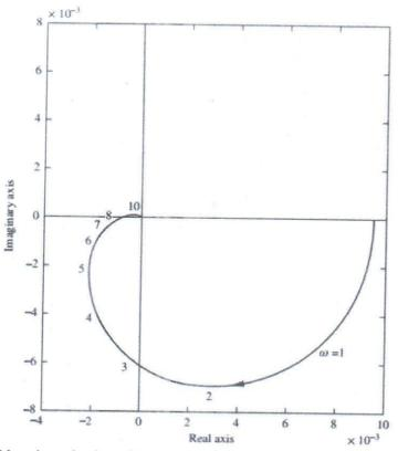
**b)** Using the Nyquist criterion, find the range of K for stability for each of the systems in the following figure.
