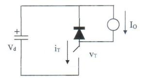
Comment on the switching power loss of the on-state and off-state of the power electronic switch. If the switching power loss increases with the switching frequency, what trade-off do you think to take for efficient switching operation?
