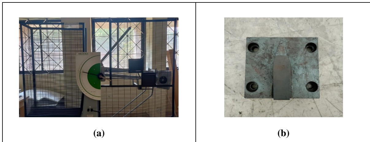
Figure 16: (a) Pendulum impact testing machine & (b) Fixture to set impact specimen.
