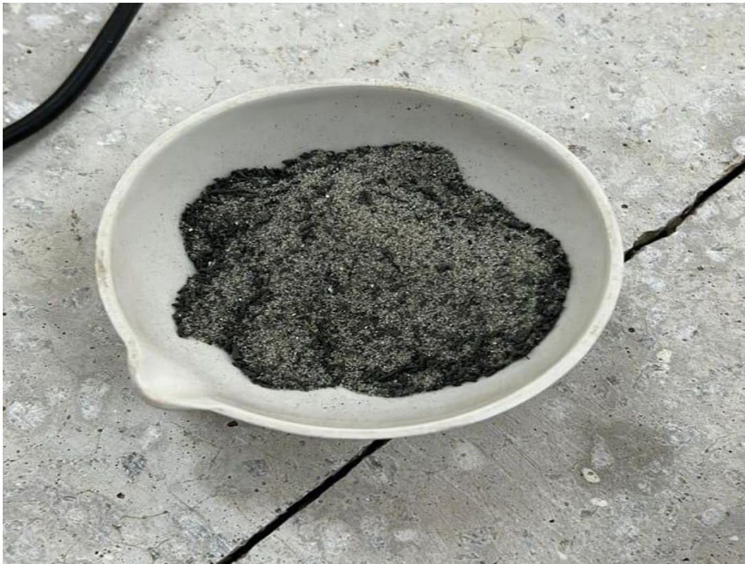
Figure 3: Sand-rubber mixture before shear test
