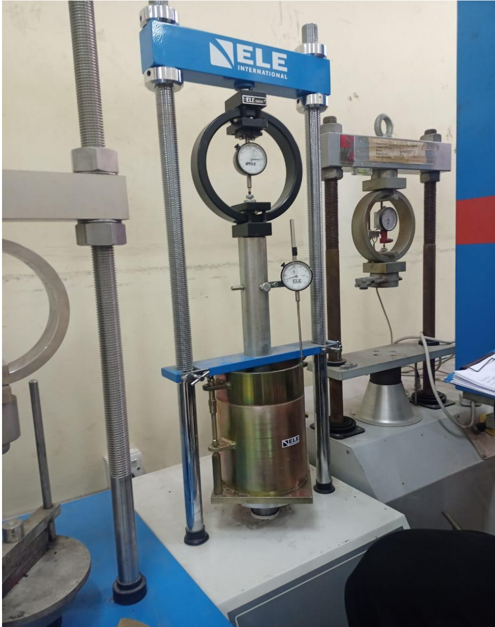
Figure 7: Performing CBR test
