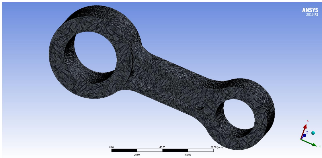
Figure 8: meshing of the connecting rod in ANSYS
