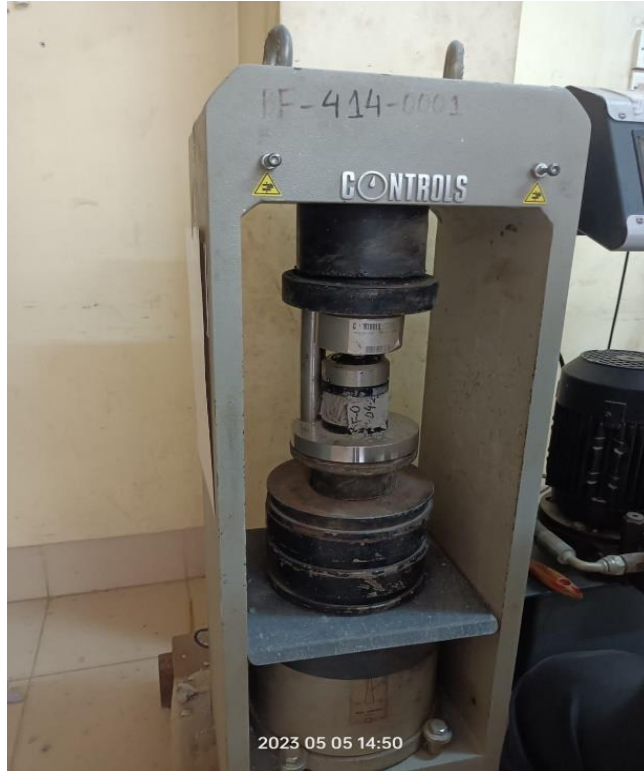
Figure 29: Cubical Sample under CTM for testing.
