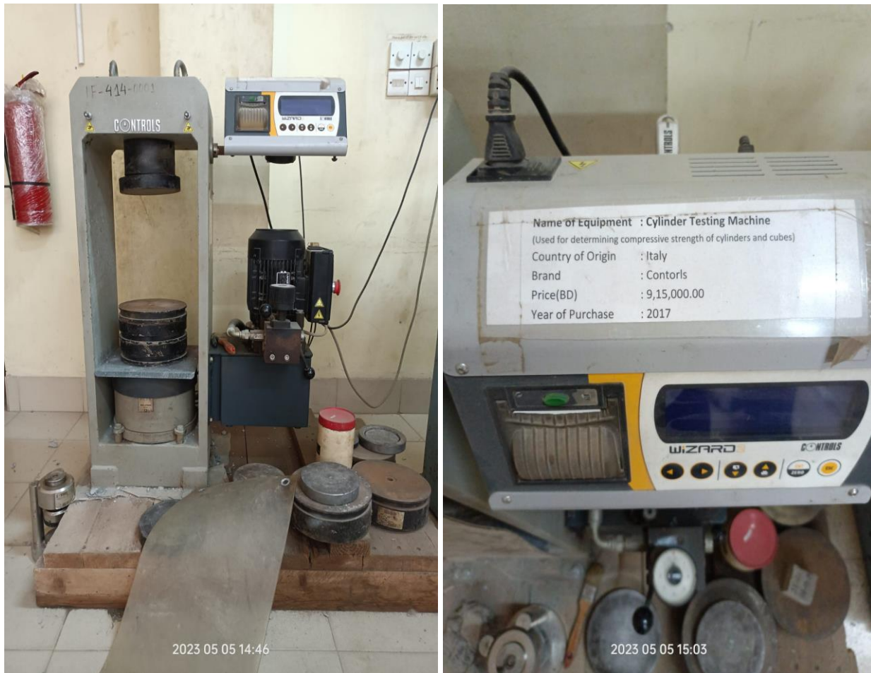
Figure 28: Cylinder Testing Machine (CTM).
