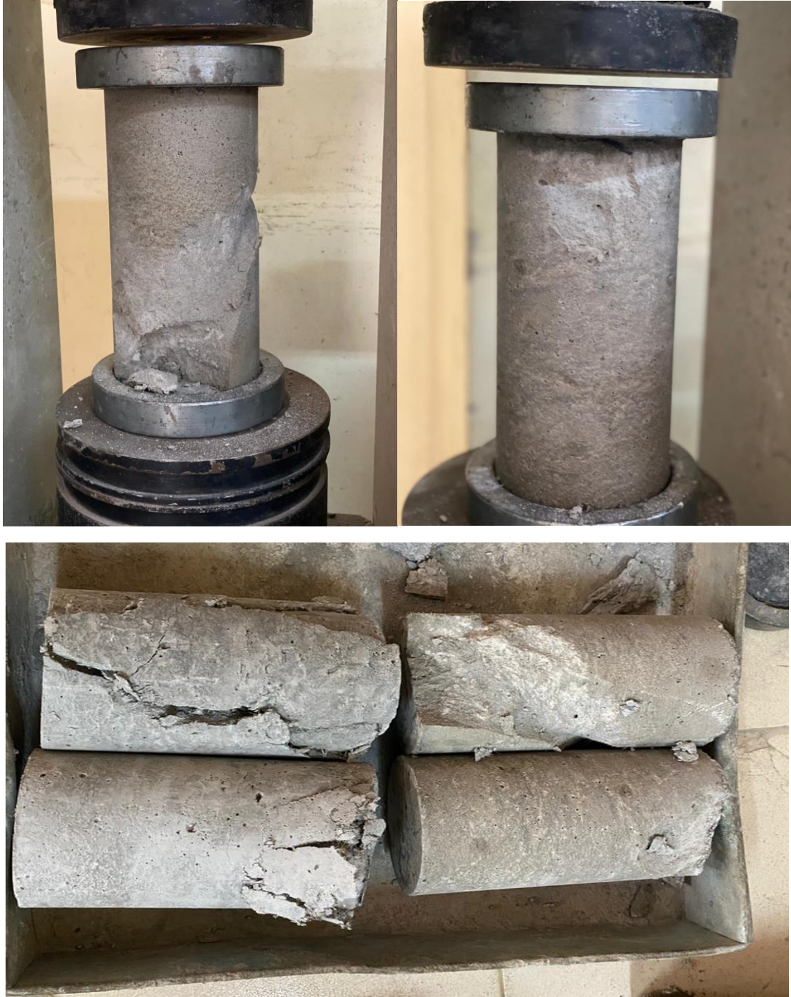
Figure 19: Failed cylinder samples from 2nd batch.
