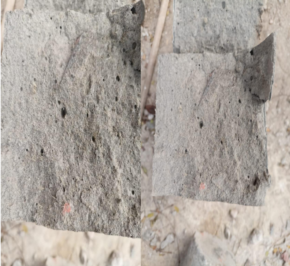
Figure 27: Breakdown of fiber bridging in beam samples.
