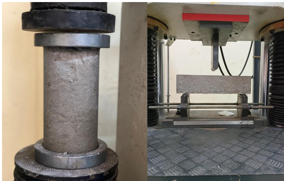
Figure 12: Samples of 1st batch under the UTM machine.
