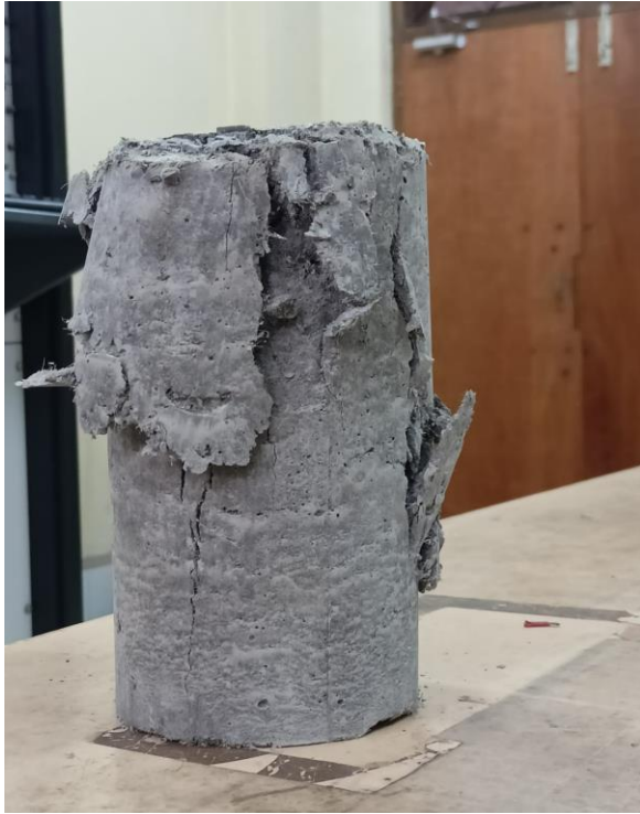
Figure 17: Failed cylinder Samples of 1st batch.
