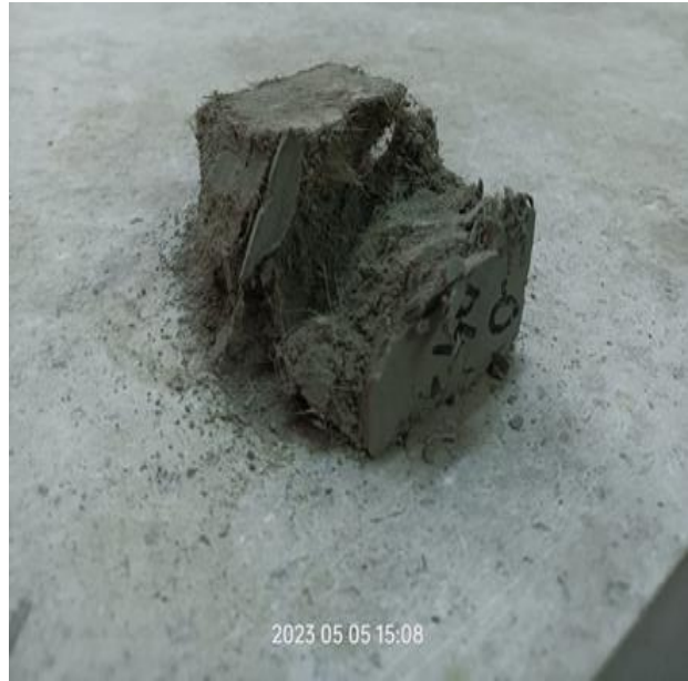
Figure 31: Failed Cubical samples of 3 to 7 batch.
