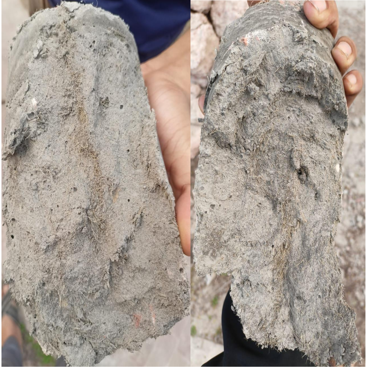
Figure 26: Jute Fiber bridging in cylinder samples.
