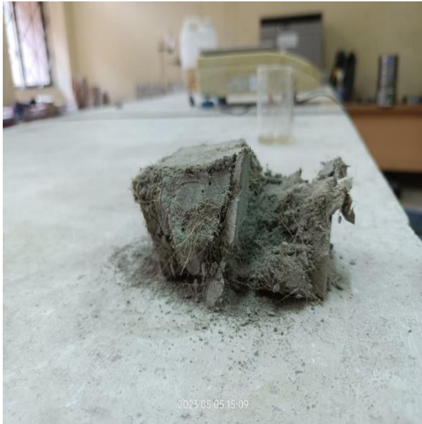
Figure 31: Failed Cubical samples of 3 to 7 batch.
