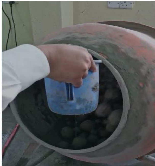
Figure 9: Casting of Jute fiber Cementitious Composites.
