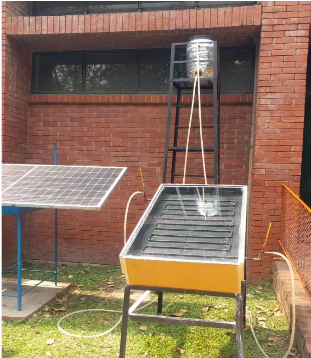
Figure 3.6: Experimental setup of the Serpentine Tube Solar Collector built at IUT, Gazipur.
