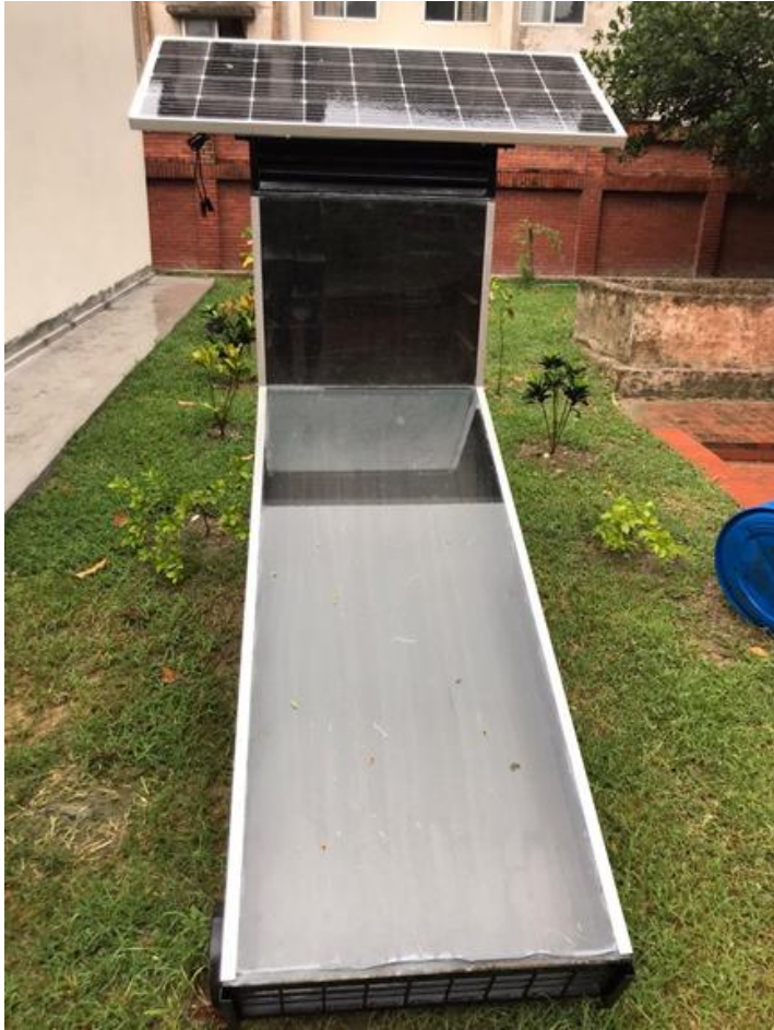
Figure 3.7: constructed solar dryer front view
