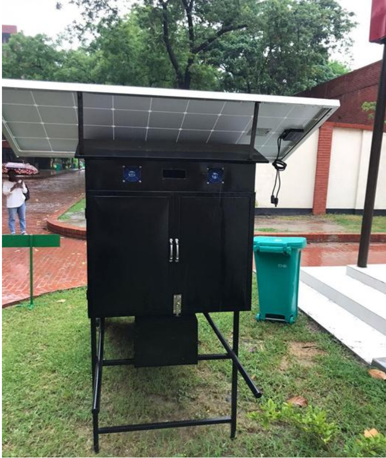
Figure 3.8: Constructed solar dryer back view
