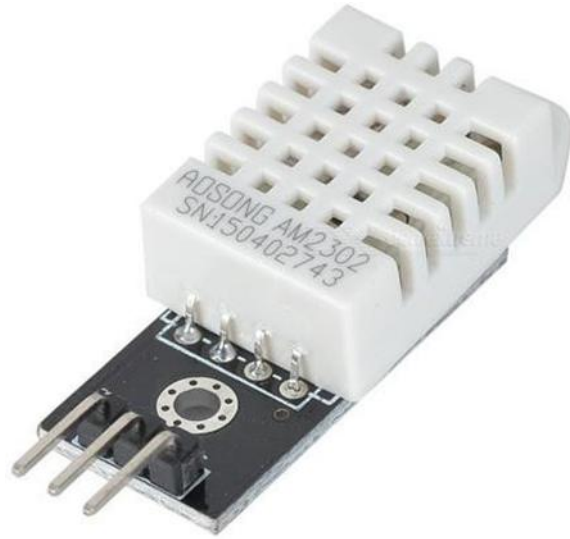
Figure 3.3: DHT 22 sensor which contains both humidity and Temperature sensor. Measuring range: temperature -40-80 °C; humidity 0; 99.9%RH. Measurement accuracy (25°C): temperature: + 0.5; humidity:+ 2%RH (10; 90%RH) Resolution: temperature: 0.1°C, humidity: 0.1%RH.
