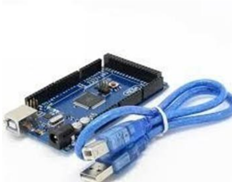
Figure 5: 54 Digital I/O terminals (14 of which have programmable PWM outputs).16 Analog Inputs.4 UARTs (hardware serial ports).16 MHz crystal clock, Robotics BD Operating voltage: 6 ~ 12v, Dimensions: 110 x 53 x 15 mm
