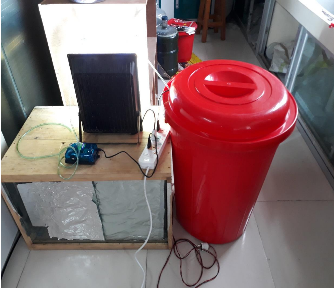
Figure 7: Lowcost Photobioreactor setup
