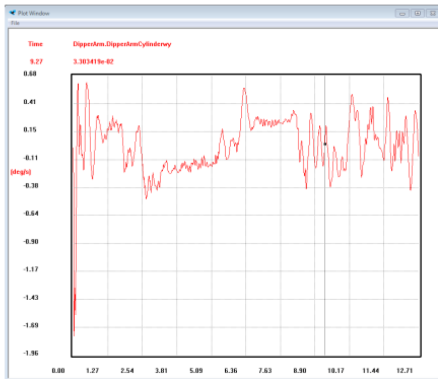
Figure 3. 8 The values of the cylinder-piston velocity of the dipper arm in a small hydraulic circuit
