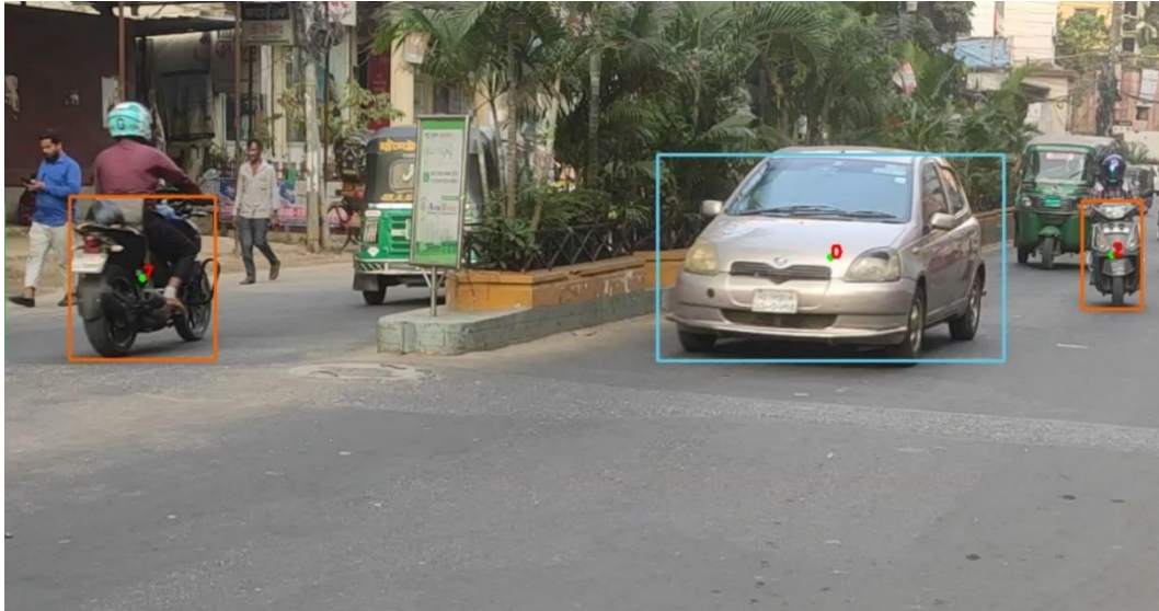
Fig. 3.24: Different class vehicles given different color BB
