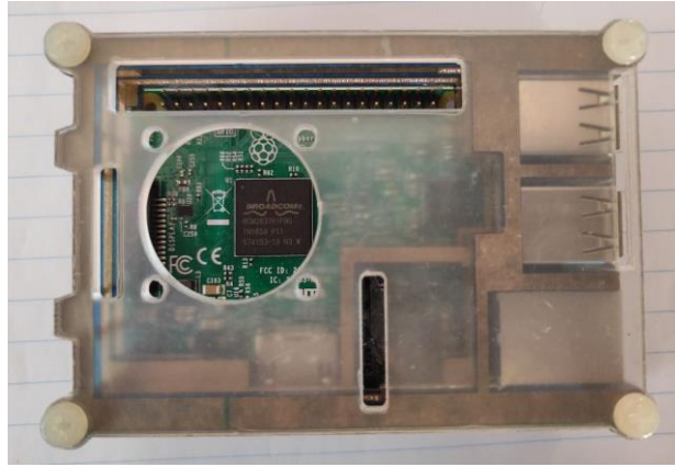
Fig. :1.6: Physical image of a Raspberry Pi (mini-computer)
