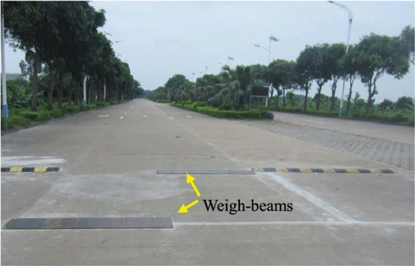
Fig. 2.1: Invasive: Weigh beams installed into the pavement [17]
