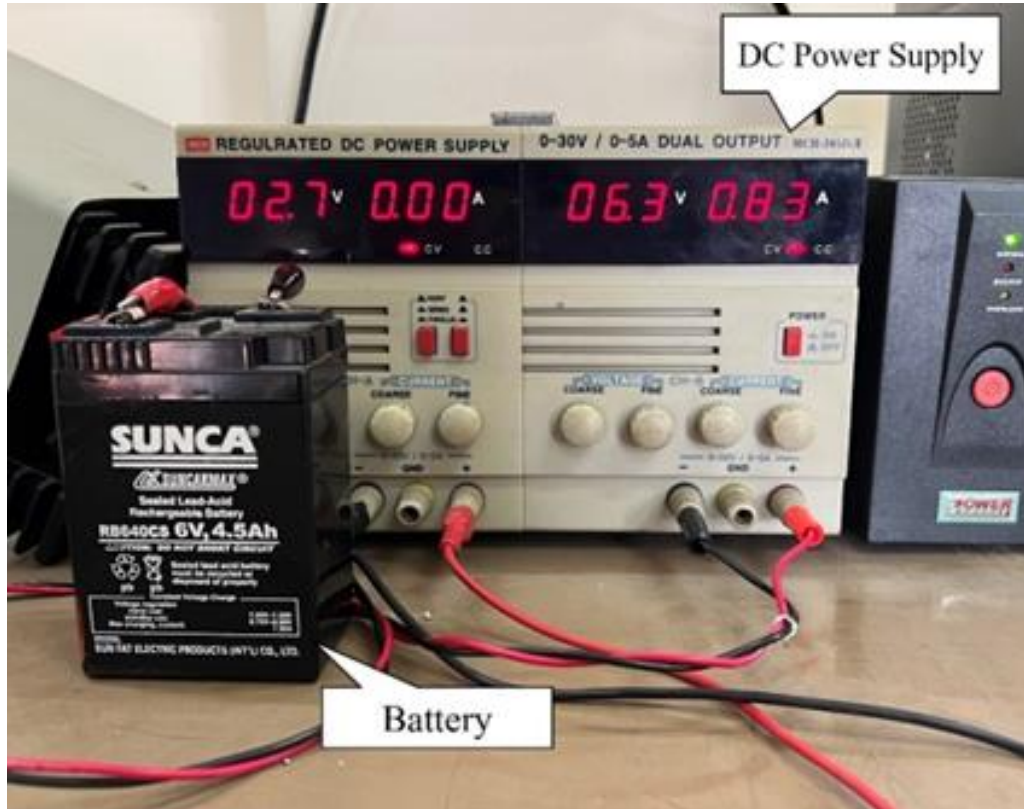
Figure 3.4. Experimental Setup for DC charging
