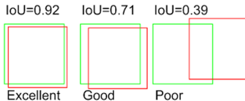
Figure 4.2: Intersection Over Union used in YOLO
