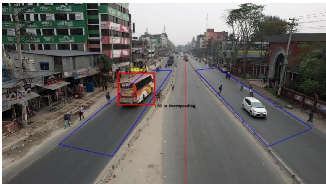
Figure 5.3: Performance of over-speeding detection
