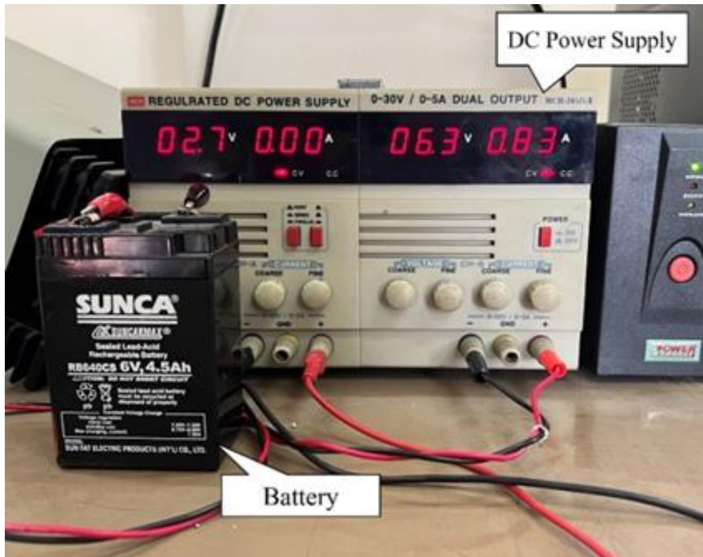
Figure 3.4. Experimental Setup for DC charging
