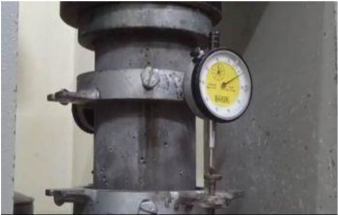
Figure 15: Strain measurement using dial gauge
