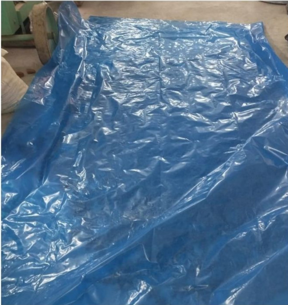
Figure 2: Coated aggregates covered with polythene
