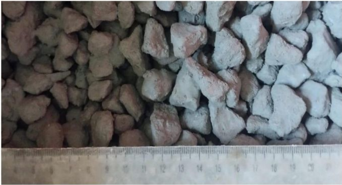
Figure 7: Fly ash and lime double coating
