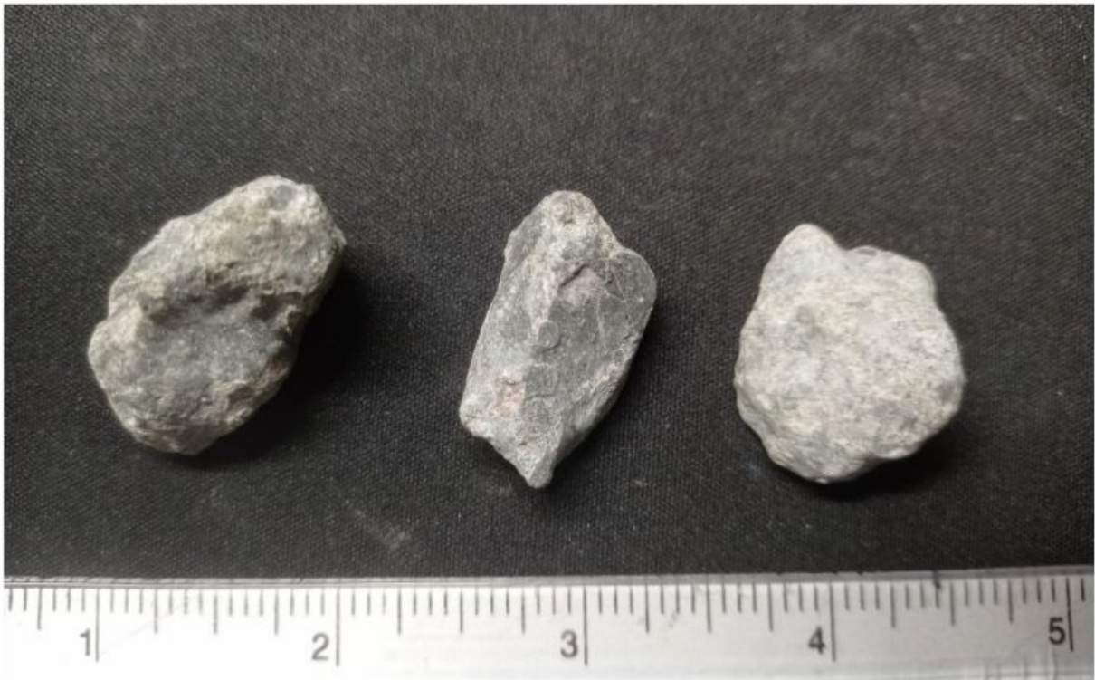
Figure 5: Cement double coating
