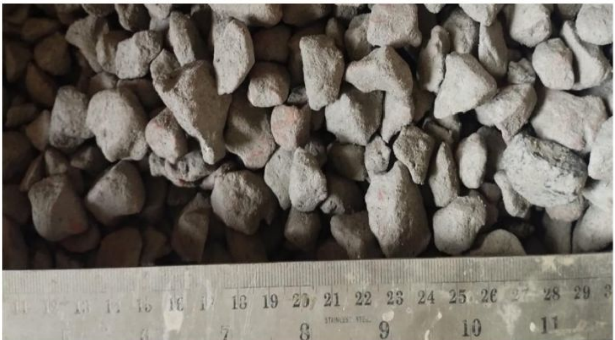
Figure 6: Fly ash and lime single coating
