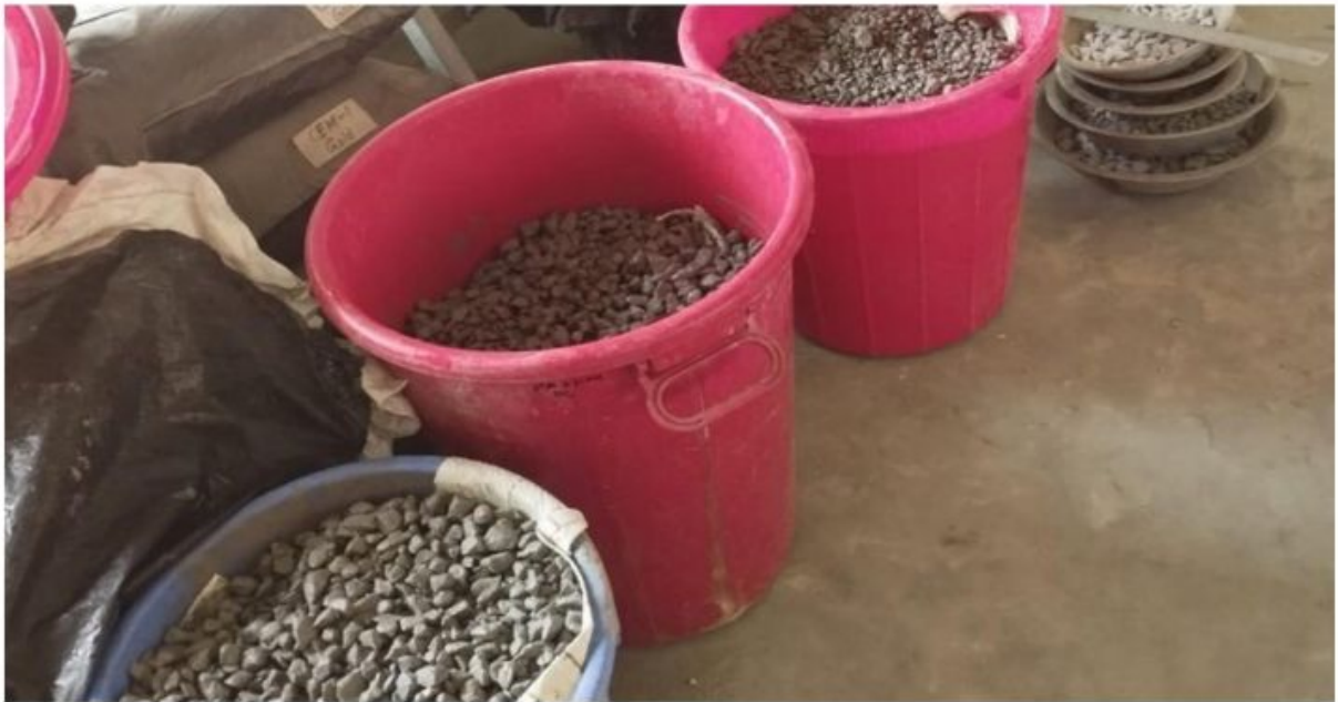
Figure 3: Coated aggregates stored in buckets
