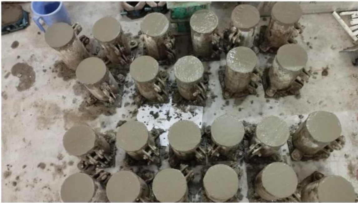
Figure 11: Casted cylindrical specimens
