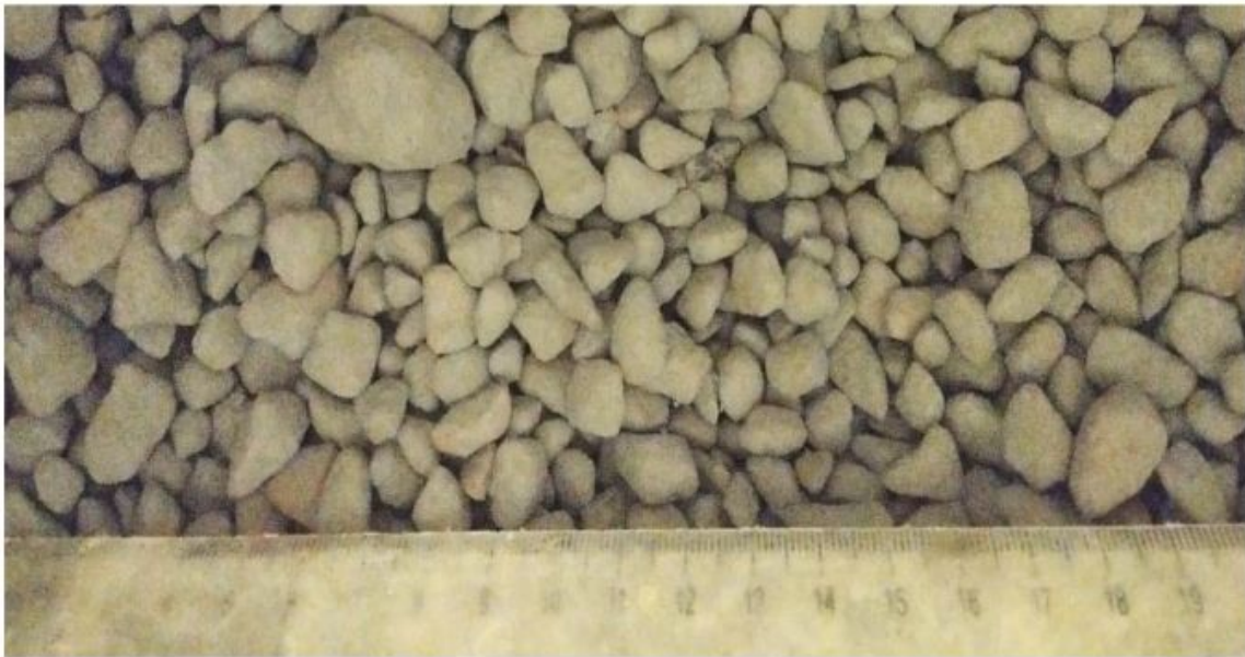
Figure 9: Slag and lime double coating
