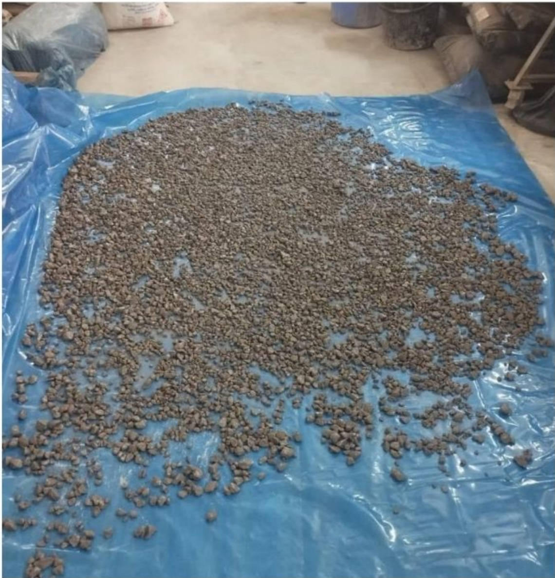
Figure 1: Coated aggregates spread over polythene
