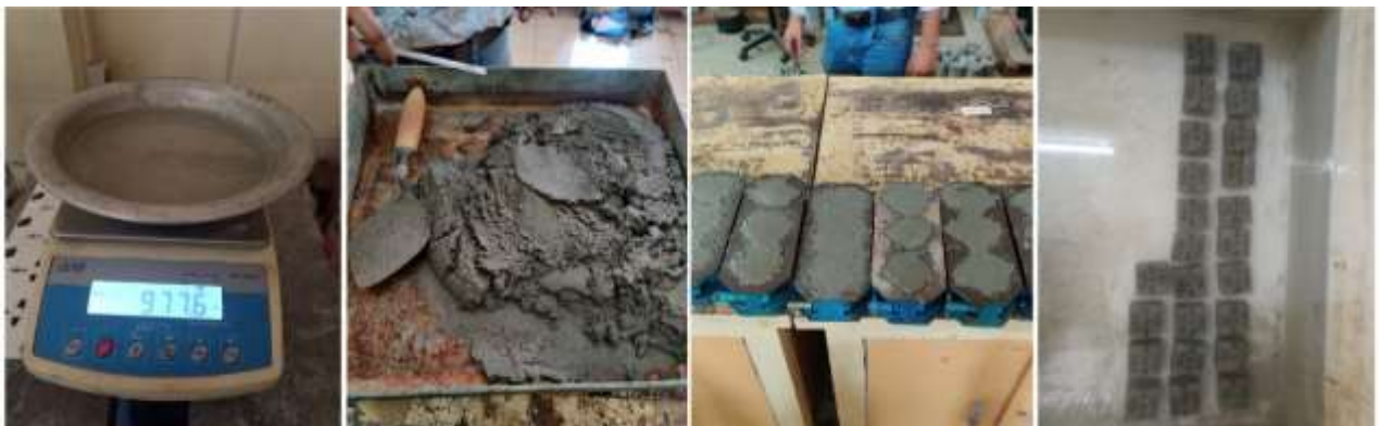
Figure 3-5: Mortar Casting & Curing Procedure
