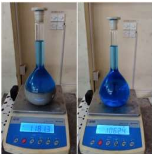
Figure 3-3: Specific Gravity Test Procedure
