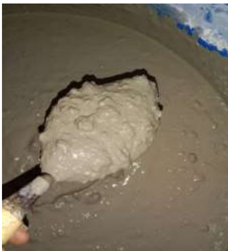
Figure 3-2: RCSW from RMC Plant
