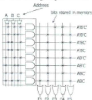
Figure 3: Programmable logical array (PLA) circuit.
