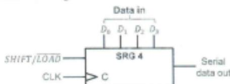
Figure 2: Logic symbol for 4-bits PISO SR.
