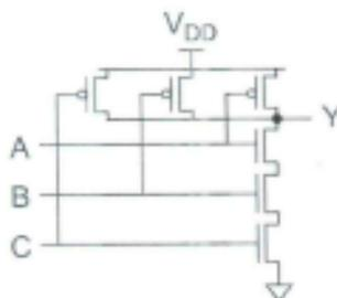
Figure 1: NAND logic circuit with three inputs.
