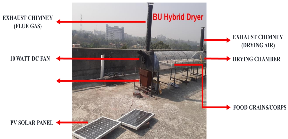
Figure 10: Solar-Biomass Hybrid Dryer
